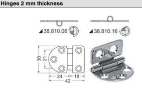
Made of mirror polished stainless steel. Vibration damping by means of a braked central axle.
