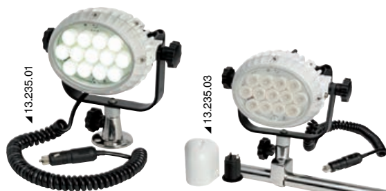
Characteristics: - Made of white painted aluminium + ABS + stainless steel base. - 13 x CREE genuine high-quality LEDs , 50,000 hour lifetime. - Light can be removed from the base thanks to the 2-m extension cable. - Fitted with watertight ON-OFF switch and watertight end plug, for either external or built-in installation.
