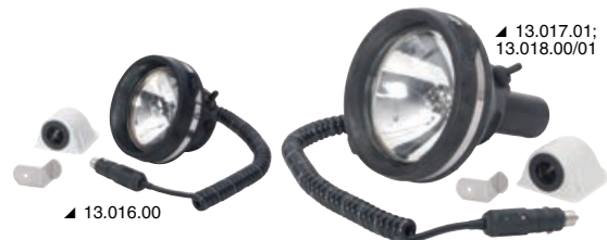
Supplied with GE watertight bulb, fitted with extensible cord, length 2.5 metres. It includes watertight plug, socket and AISI 316 stainless steel bracket for wall-mounting installation.
