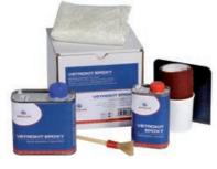
65.520.10 For fiberglass repairs. Made of epoxy resin + catalyst, 500+250 g, mixing container, sandpaper, gloves, 50x50-cm glass fibre cloth, brush and broad knife.
