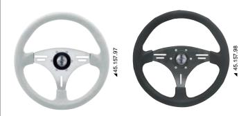
Anodized aluminium spokes and soft polyurethane crown.
