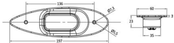
**Evolo low consumption LED navigation lights made of stainless steel for flat mounting**
